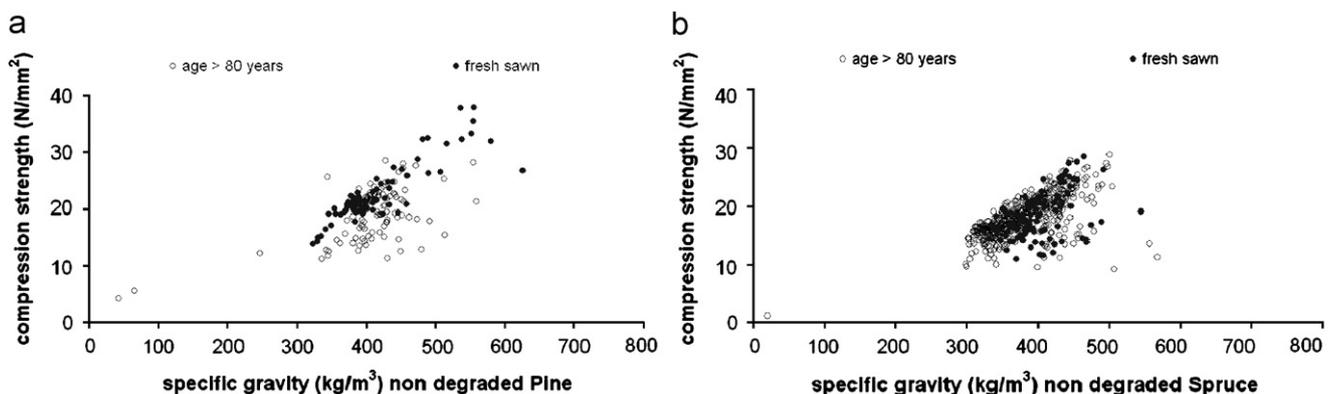
Fig. 7. Comparison of relationship between compression strength and specific gravity in piles that are >80 years in service and freshly sawn material for pine (left) and spruce (right).
