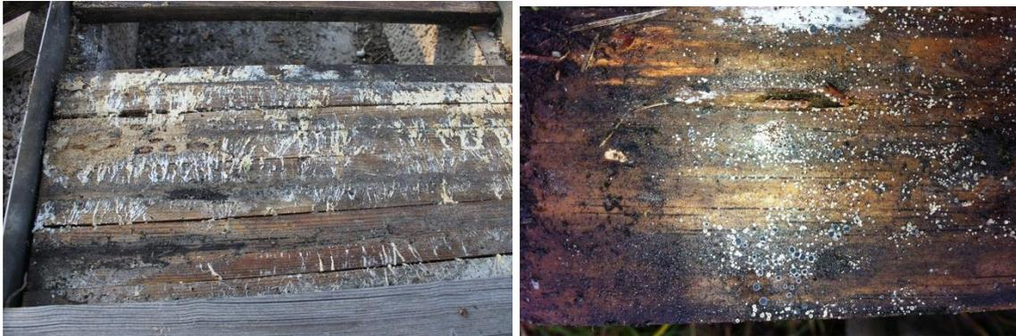
*Figure 4. Decay in TMT-UC2 stakes in deck in Italy and Control stakes in deck in Denmark after 6 years.*
