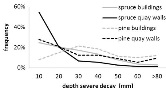
Fig. 11. Frequency diagram of the depth of severe decay in spruce and pine piles under buildings or quay walls.
