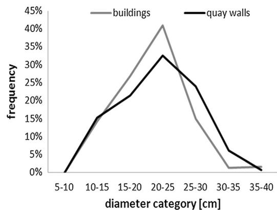
Fig. 2. Frequency diagram of the pile head diameter.
