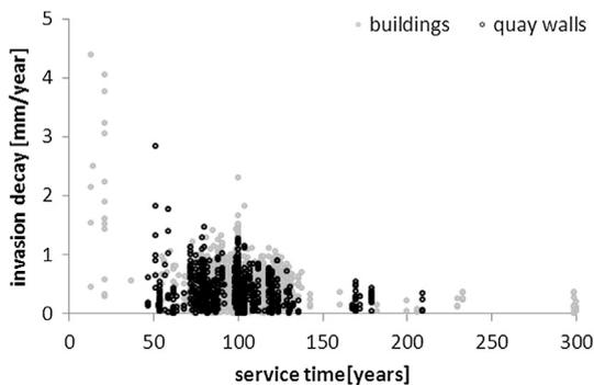
**Fig. 8.** Velocity of bacterial invasion in piles under buildings and quay walls in relation to service age.
