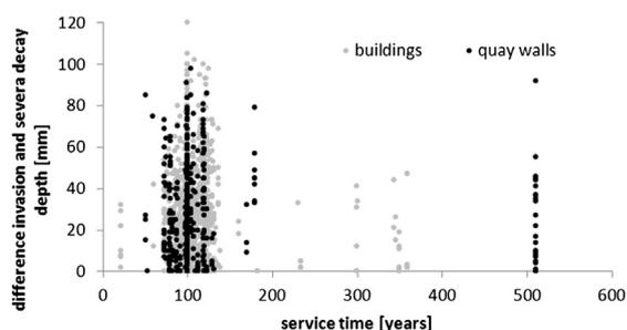
Fig. 12. Activity of decay in pine piles under building and quay walls in relation to service age.
