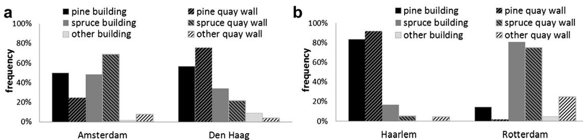
Fig. 4. Frequency diagram of the occurrence of timber species of piles under buildings or quay walls in and soil in Amsterdam, Den Haag, Haarlem and Rotterdam.
