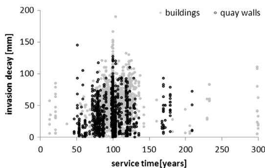
Fig. 6. Depth of bacterial invasion in piles under buildings and quay walls in relation to service age.
