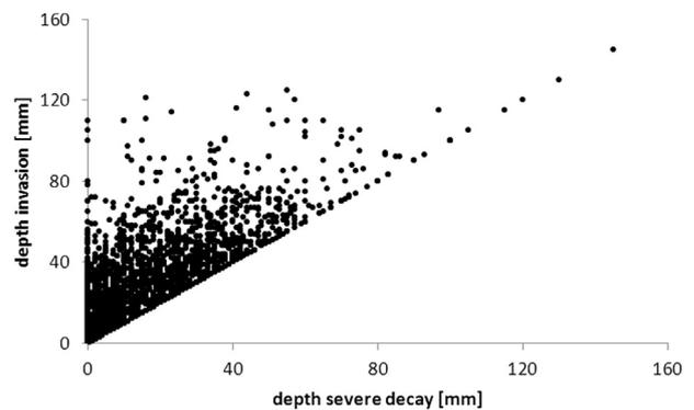
Fig. 16. Relation between thickness of depth of bacterial severe decay and invasion in spruce ( $N = 1880$ ).
