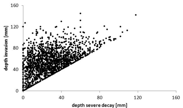
Fig. 17. Relation between thickness of depth of bacterial severe decay and invasion in pine ( $N = 1859$ ).
