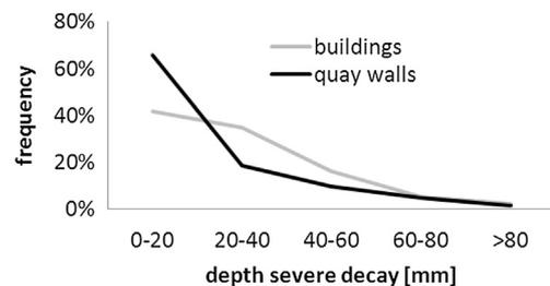
**Fig. 10.** Frequency diagram of the depth of severe decay in piles under buildings or quay walls.
