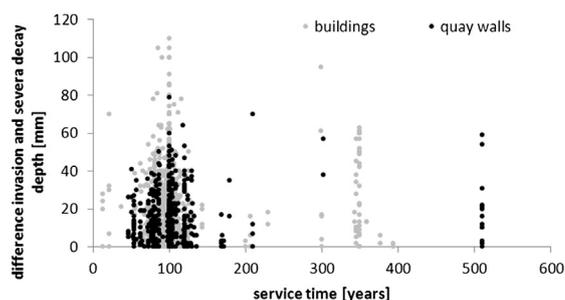
Fig. 13. Activity of decay in spruce piles under building and quay walls in relation to service age.
