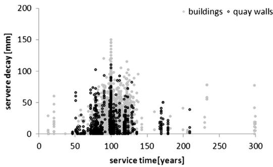
**Fig. 7.** Depth of severe bacterial decay in piles under buildings and quay walls in relation to service age.
