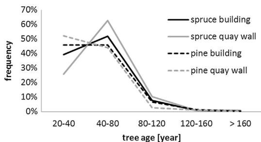
Fig. 5. Frequency diagram of the tree age of the pile head.
