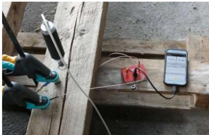
Figure 1: spotWave system (little red box) and all 3 system sensor connections (on the left)
