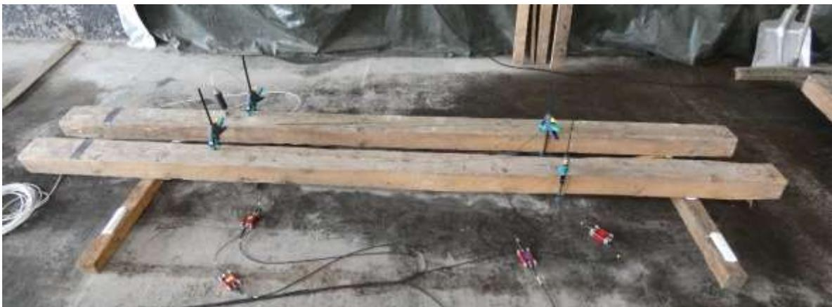
Figure 2: Synchronized measurements WWD-AMSY on beam 9 (upper left)
